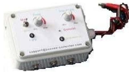
Fig. 5. An efficient power pack (stabilizer) with 25 to 50mV capacity.
